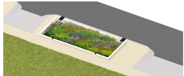
Fig 7.6: Install the specified vegetation and top dressing mulch cover
