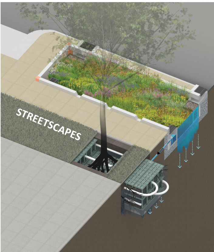
Example RAFT installation - complete assembly prior to backfill and planting.
